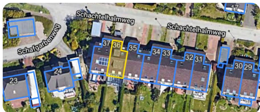
Figure 5: Buildings are recognized by an image-processing algorithm (Picture courtesy of SkenData ©)
