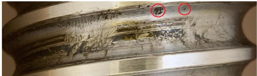
Figure 5: Example image of the KIT ball screw drive dataset - defect highlighted in red
